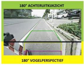
A 2-in-1 view of both the horizontal view and the bird's eye view is displayed on the LCD monitor.
